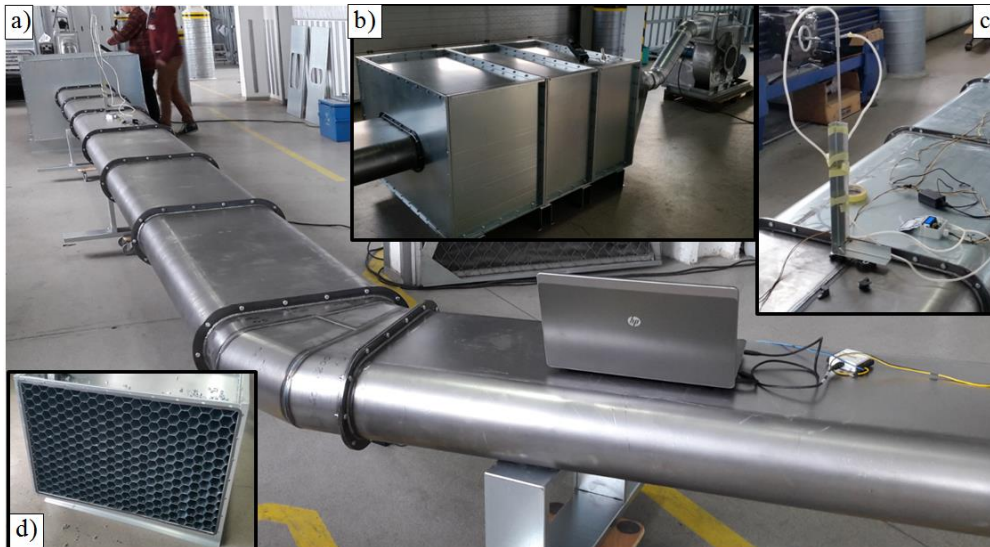
Fig. 4: Laboratory stand a) duct with supply system, b) view of supply system, c) measurement point, d) flow straightener.
