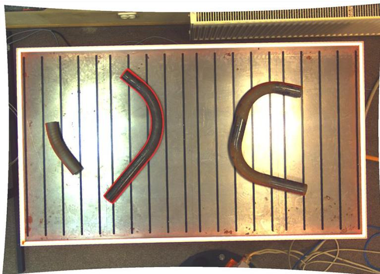
Fig. 3: The image straightened with the calibration camera model.
