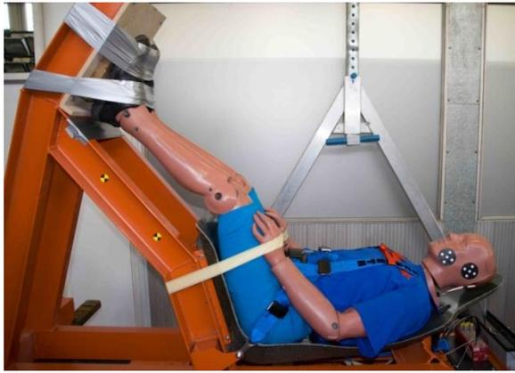
Fig. 1: Dynamic sled test with 50 % HybridII.
