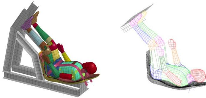
Fig. 5: Model of the test in MSC.Nastran700 (left) and in MSC.Dytran (right).
