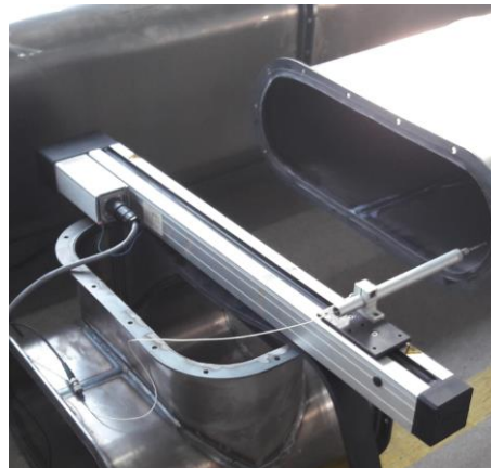
Fig. 6: Hot wire anemometer Dantec was used for velocity profile distribution measurement.
