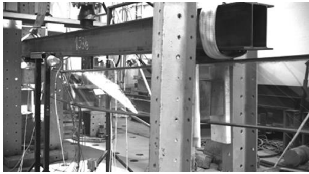
Fig. 1: Buckling of the hybrid steel-glass beam.
