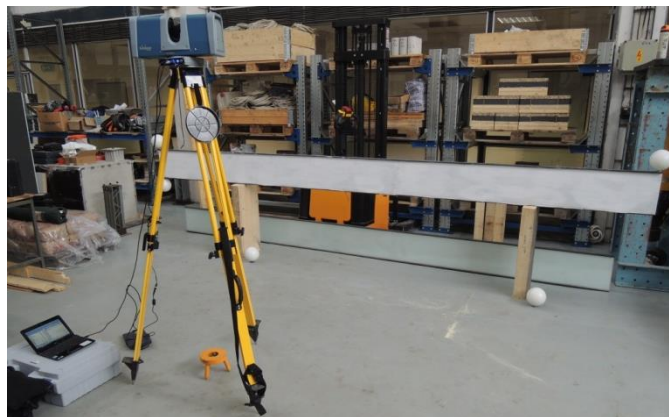
Fig. 2: Laser scanning, first standpoint.
