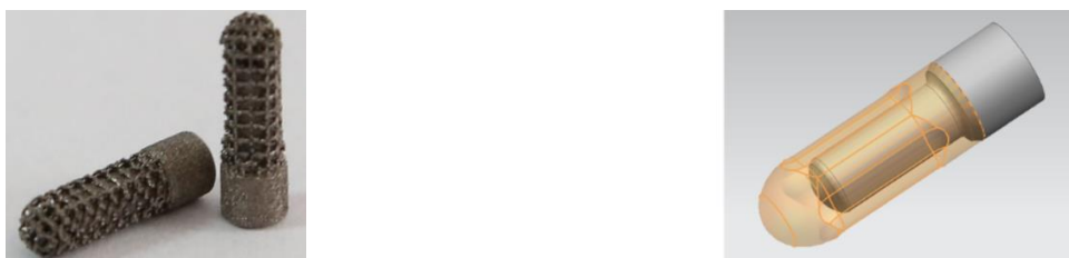
Fig. 5: Specimens (left) and structure composition (right) of the final implant for future analyses.
