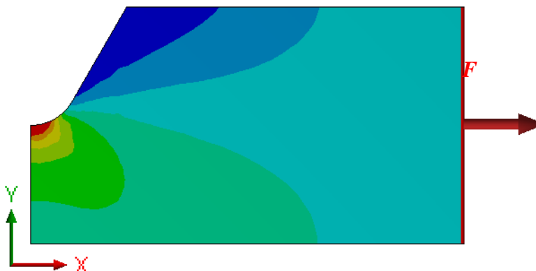
Fig. 3: Stress distribution map for the notched specimen.
