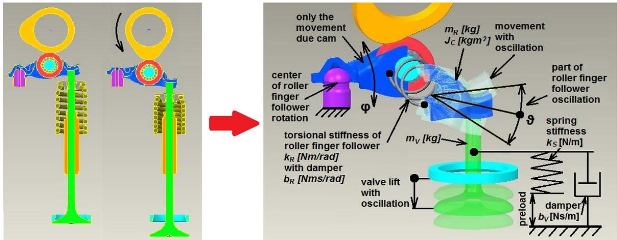
Fig. 2: Real and mathematical model of valve mechanism.
