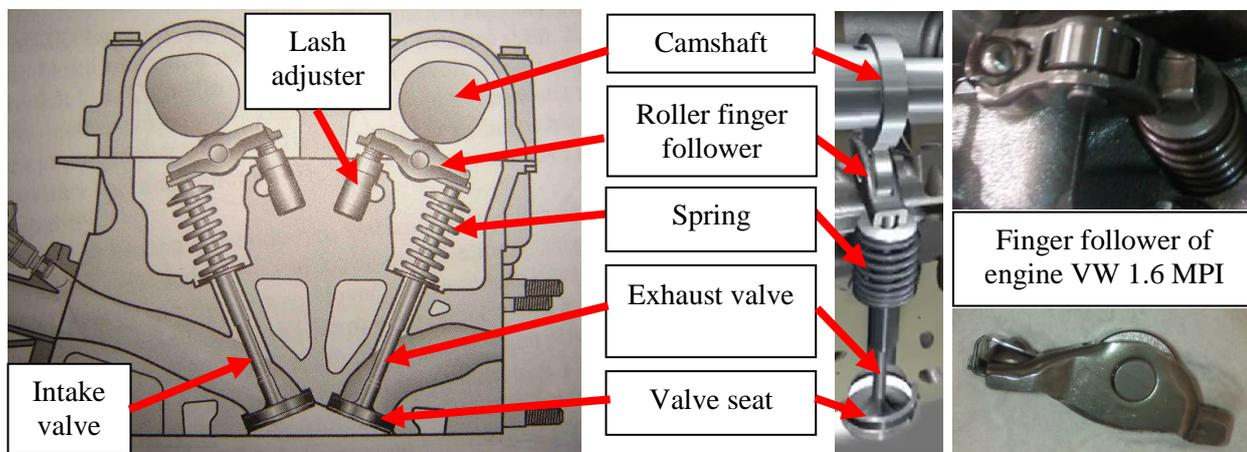
*Fig. 1: Valve mechanism in combustion engine head.*
