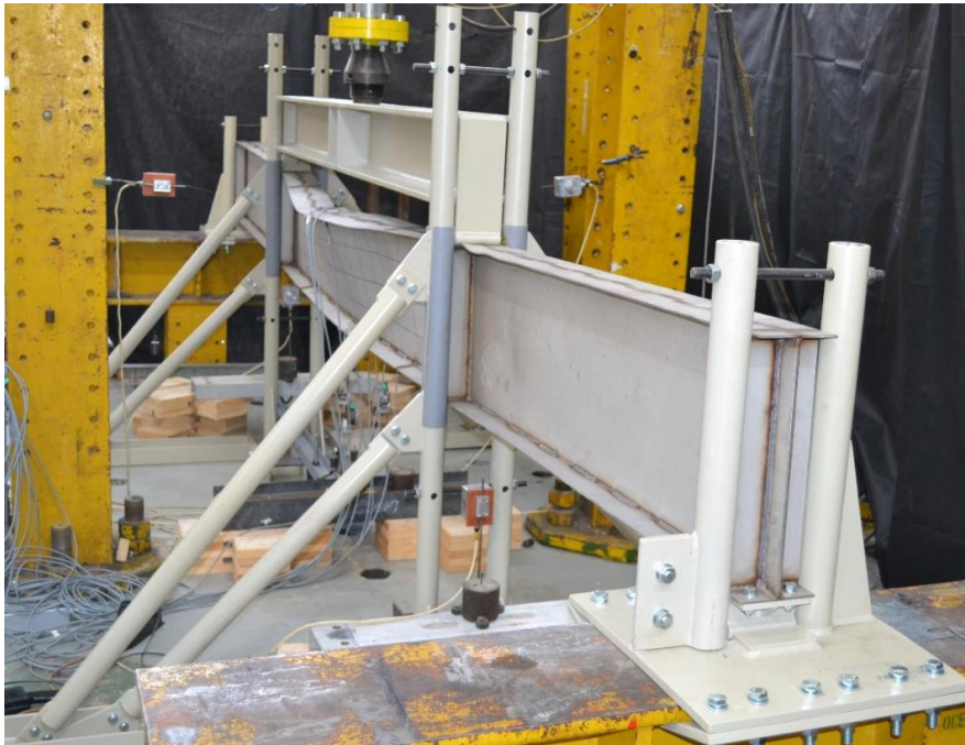
Fig. 2: Test arrangement and beam failure mode (test 1).
