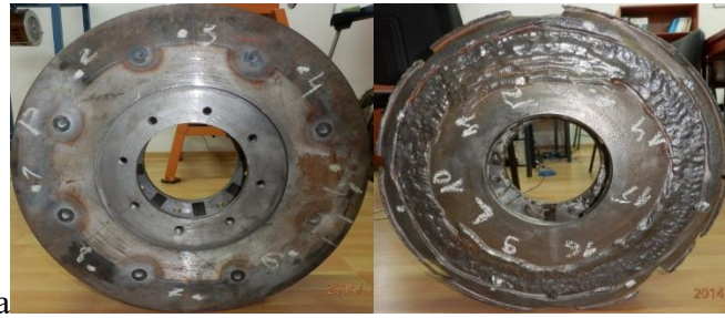
Fig. 1: Blade wheels of a projecting rotor (from left): new wheel, worn wheel.
