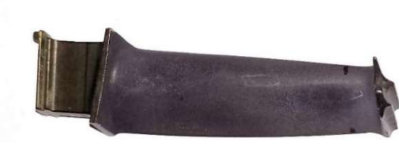
Fig. 2: The turbine blade after the service life
