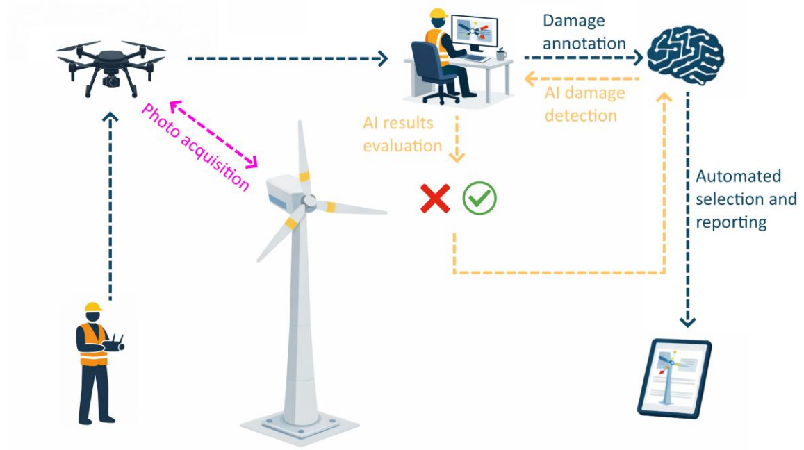
Fig. 1: Workflow of the proposed UAV-based inspection and YOLOv8-assisted damage detection framework for wind turbine blade condition assessment.
