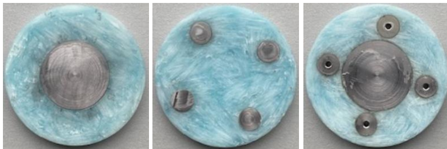
Fig. 4: GFRP with bonded-in steel drill bushings.
